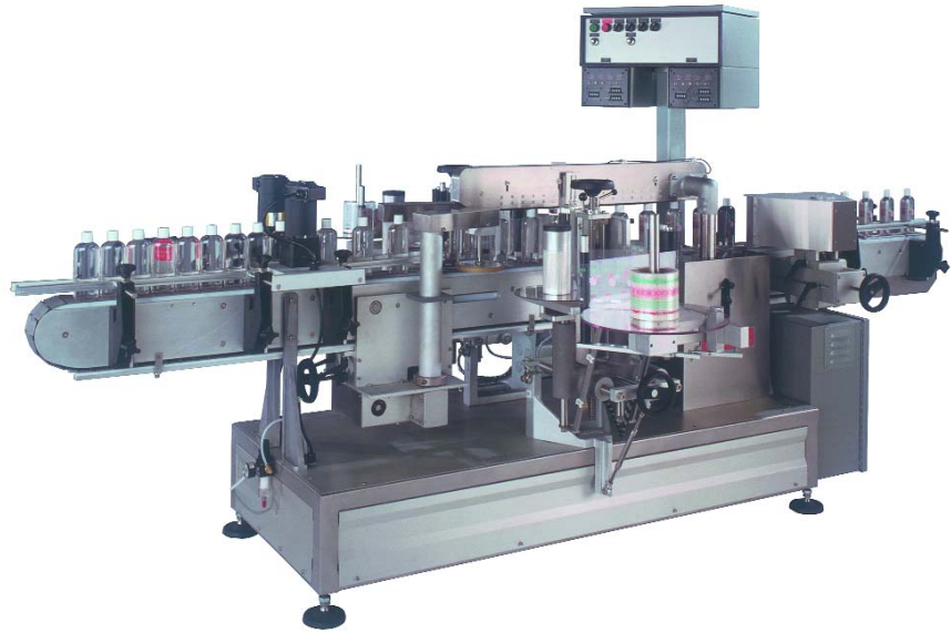
Accraply's 35PW Panel & Wraparound Labeler features stepper-driven label applicators with ratio-offset and speed following capability, plus adjustable variable-speed conveyor.
